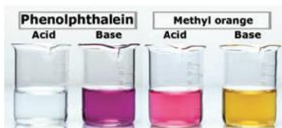
Figure 14.4 Test for acid and base using indicator
