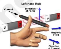
The law states that while stretching the three fingers of left hand in perpendicular manner with each other, if the direction of the current is denoted by middle finger of the left hand and the second finger is for direction of the magnetic field then the thumb of the left hand denotes the direction of the force or movement of the conductor.
